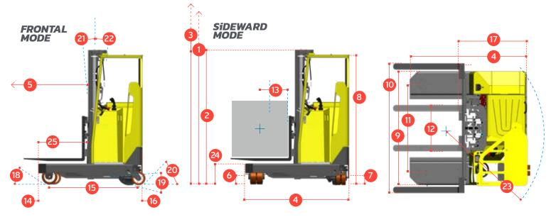
This compact truck features one rear wheel drive with a large rubber tyre and 360° steering rotation. The multi-functional controlled joystick allows the operator to change direction and travel speed in a smooth seamless motion, in addition to full control of all the hydraulic functions. This contributes to faster procedures for manufacturing distribution and logistics operations.
